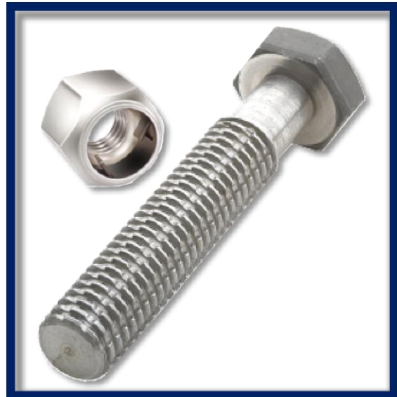
A TineLok vibration-proof fastener showing longitudinally grooved bolt alongside the nut with locking "tined" insert
